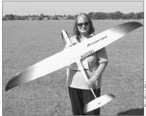
Erica Pike, Team Oz helper, chief cook and bottle washer and trainer of the Oz cheerleader team, keeps Ray's batteries warm in one of his Surprise XI+'s. Model uses a Plettenberg F5B 10 motor with 7:1 g'box, a Schulze 18.149/199 controller and RFM 17x18 prop. Pack is 17 or 18 cell GP3300's. The prop is installed on a +7° hub, making it a 17x24! Ray says this setup works well on both 10 and 18 cell packs
