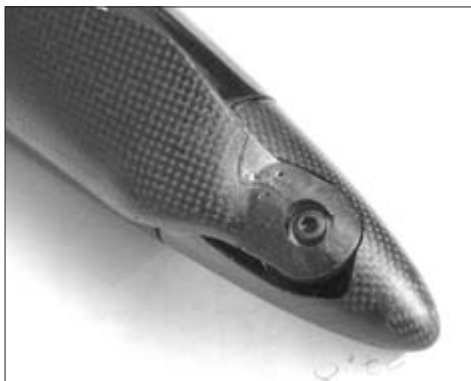
The clever prop/hub/spinner design used on the Italian models to reduce drag with the blades folded.
