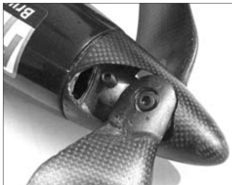
The clever prop/hub/spinner design used on the Italian models to reduce drag with the blades folded.
